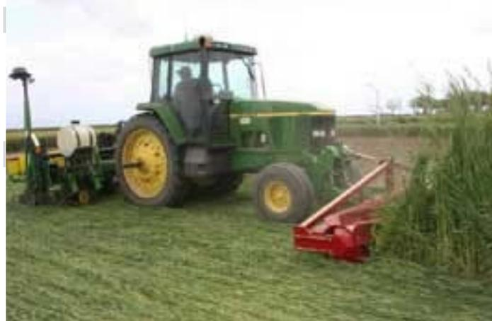
Using a roller-crimper to terminate headed out cereal rye
